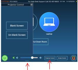
3.) You can adjust the volume by adjusted the Volume Control. Also you can mute or unmute the projector by tapping on the Projector Control button and then tapping on the Blank Screen or Un-blank Screen.
