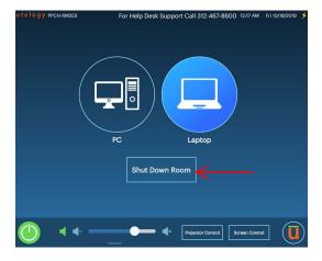
5.) You can shut off the classroom equipment by tapping on the Shut Down Room button.
