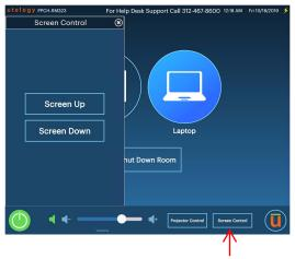
4.) You can raise or lower the projector screen by tapping on the Screen Control button. and then tapping on the Screen Up or Screen Down.
